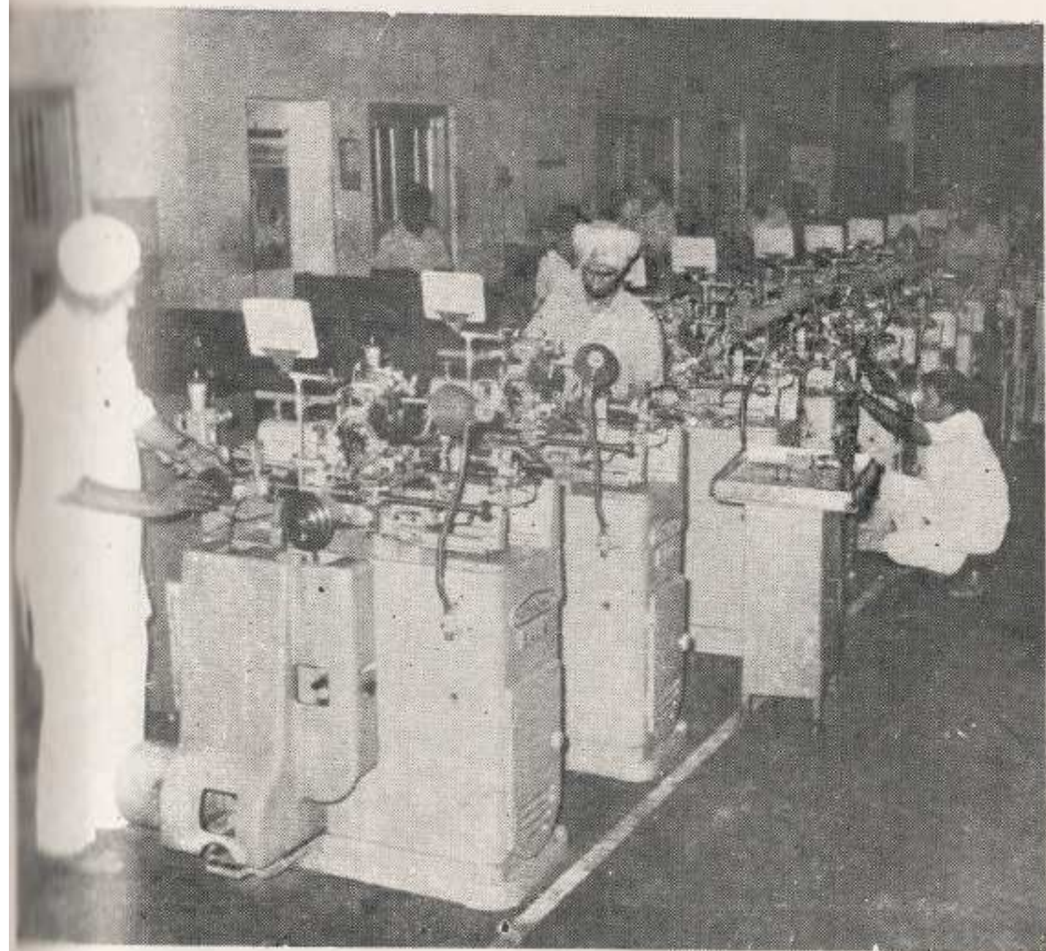
The Creator beside his proud creation. S. Karam Singh Bhogal standing beside the row of the Turn-O-Mat sliding head-automatic lathes.
