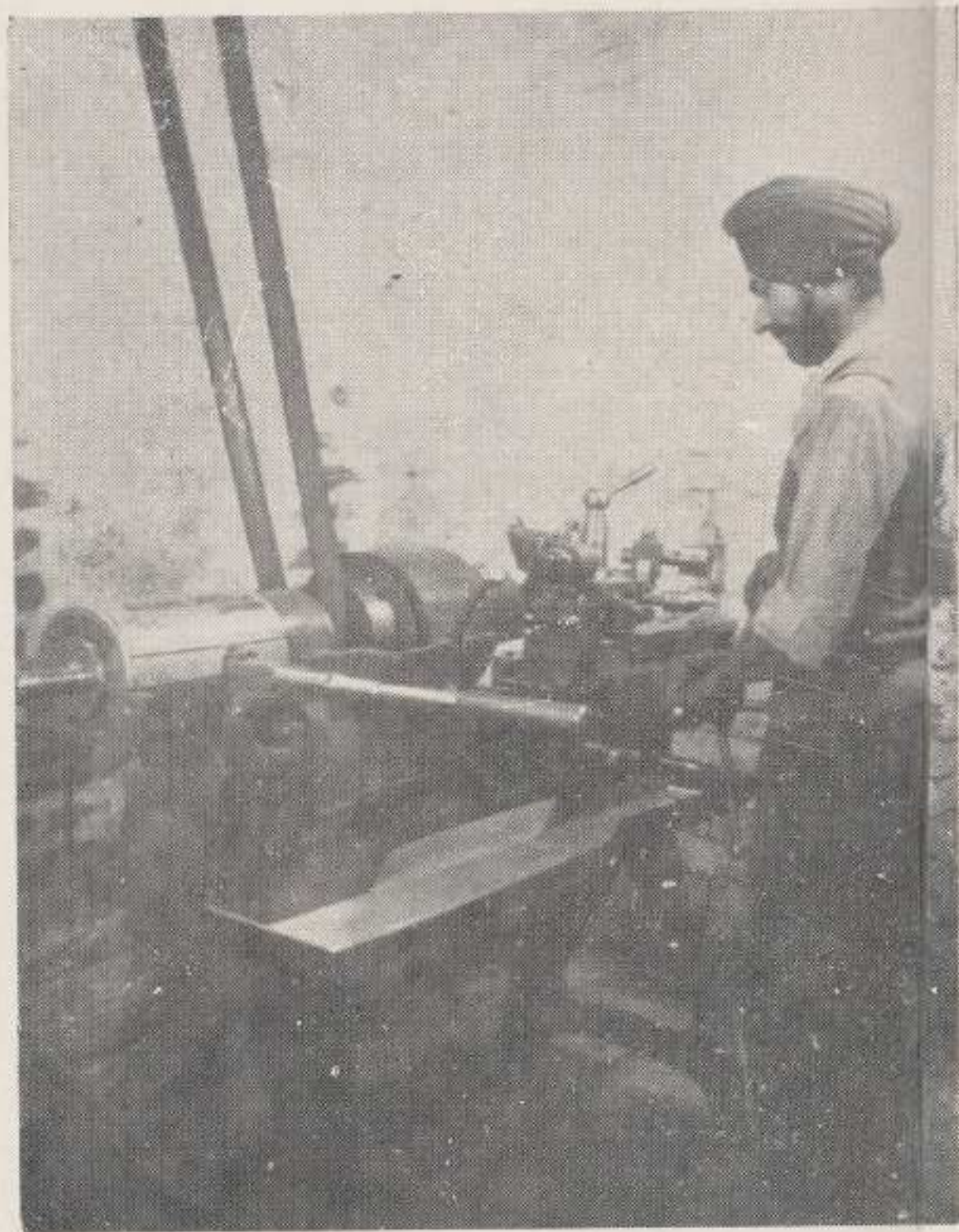
S. Mohinder Singh Bhogal working on the Company's first self-designed and manufactured Capstan Turret Lathe.
